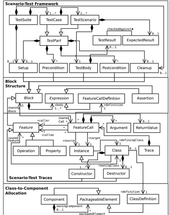
Figure 4: Test-execution metamodel including scenario-test framework (STF;[35]), internal test-block structure, scenario-test traces [16], and class-to-component allocation.
