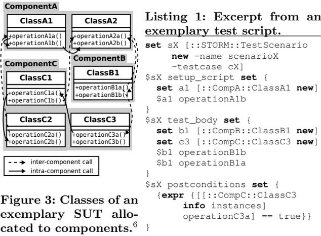
Figure 3: Classes of an exemplary SUT allocated to components.<sup>6</sup>
