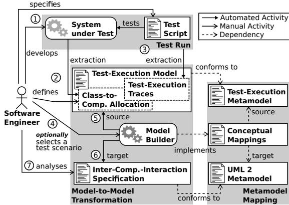
**Figure 1: Conceptual overview of deriving test-based inter-component-interaction specifications.**
