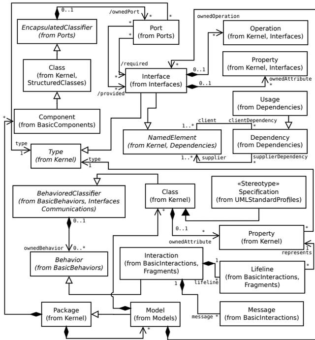
**Figure 5: Selected elements of the UML2 metamodel [27] for specifying inter-component interactions.**
