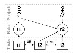
Figure 2. Example of a process-related RBAC model
