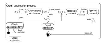
Figure 4. UML model of a credit application process
